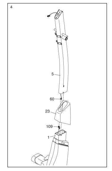
5. **Tip: Avoid pinching the wires.** Insert the Upright (5) into the Frame (1).
